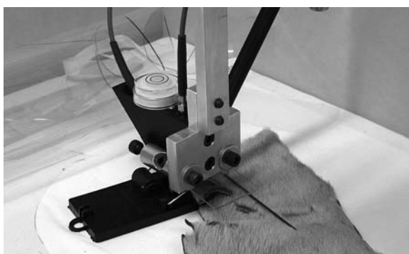
Figure 7. Testing thylacine hair clamped under glass using a modified mousetrap.
